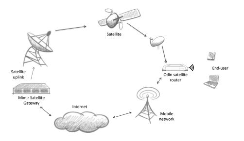
Overview of the Forsway solution. The Mimir server routes the Internet traffic over the satellite or cellular/terrestrial network, depending on traffic type, to the end-user equipment Odin.
