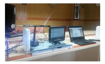
Internet over DVB-T2. The white box to the left in the picture is the hybrid modem Odin with a WiFi hotspot. The modem is connected to a low cost indoor TV antenna. 2 Mbps was measured about 7 km from the TV tower. Higher downlink speeds can be achieved with additional DVB-T2 channels.
